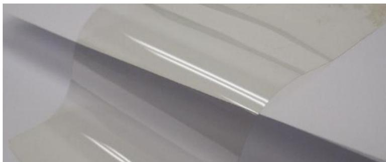
Flexible 38  $\mu\text{m}$  film produced with SD1100P-ODA
