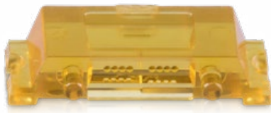
Optical interconnect lens designed and produced by Nalux Co., Ltd.
