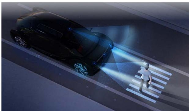
The digital matrix LED headlight could project safety or warning images in front of a car to improve safety and security for both drivers and pedestrians.
