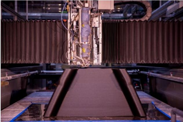
THERMOCOMP AM compounds based on amorphous resins such as ABS, PPE, PC, and PEI exhibit good creep behavior versus semi-crystalline resins, and reduced deformation under constant pressure. Further, lower shrinkage during cooling means these materials demonstrate greater dimensional stability and less thermal expansion during part use.
